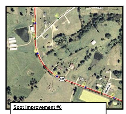
Widen lanes and shoulders through this 40 MPH curve to current standards and soften curve radius. (Trimble MP 0.20 to 0.60)
